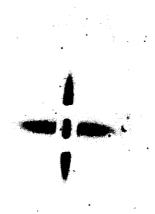
Fig. 77. Small-angle pattern from a single crystal of an Al-Cu alloy (4 per cent Cu by weight). The [100] axis is parallel to the incident beam and normal to the film, and the [010] axis is vertical. Mo K $\alpha$  radiation; sample-to-film distance, 4 cm. Enlarged 2×.
